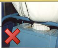
Enzyme granulates must be kept intact to avoid the release of enzyme.
